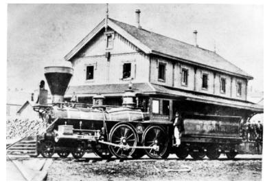
The only known photograph of a B&O loco is this undated shot of an apparently new engine in front of Brockville B&O station. The un-numbered loco appears to be named RENFREW. Donald McQueen, co-author of *Constructed in Kingston*, has identified the builder's plate (seen between the driving wheels) as one used by Canadian Engine & Machinery Co. between 1876 and 1888. Only one B&O locomotive was acquired in that time frame, so *Renfrew* is almost certainly No. 11 and the photo dates from 1877.
