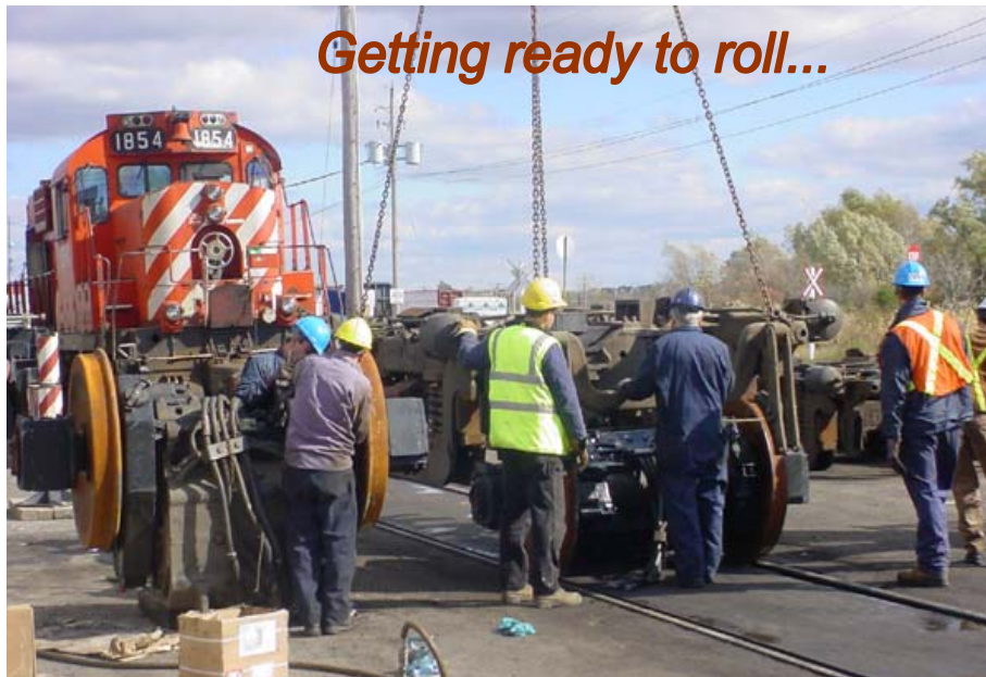
Photo: Dave Watts Wheel change-outs take time and patience. In mid October, OCR Alco 1854 gets a new set of wheels under the watchful eye of Shop Manager, Roy Murray.
