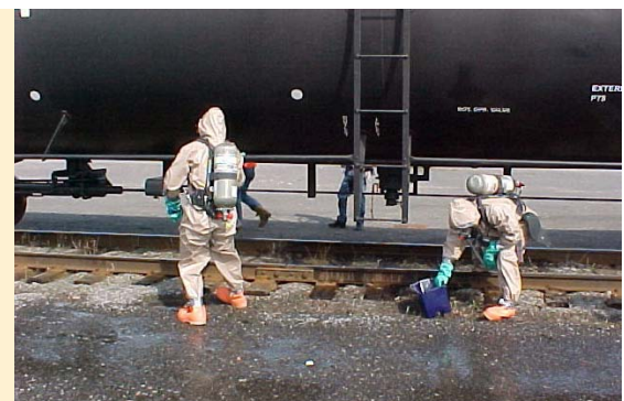
(left) "...Initial rescue of injured employee" and at right, E.R. Team closed the leaking bottom outlet valve.
